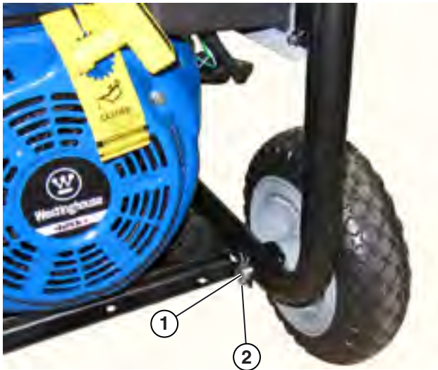
Figure 6 – Assemble Wheels to Frame
