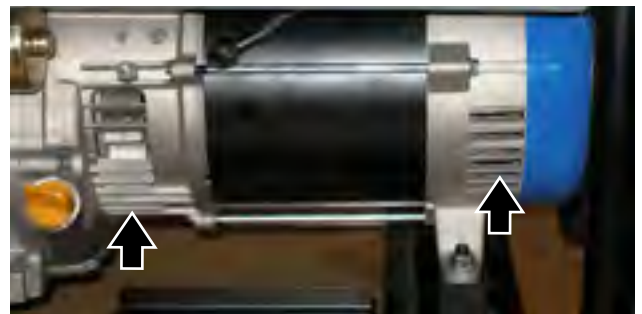
Figure 45 – Alternator Cooling Air Inlet and Outlet Port
