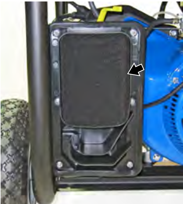
Figure 31 – Removing Coarse Outside Air Filter
