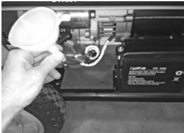
Figure 28 – Adding Engine Oil
